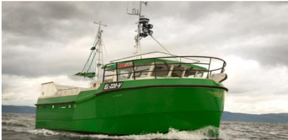
Figure 5: Hybrid fishing vessel in Norway reducing CO 2 emissions by up to 70% (EA Energianalyse, 2023a)
