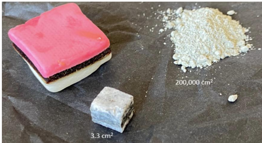
Figure 11: Glacier flour (powdered material) has a very high surface area. The larger contact surface is the reason why the reaction with CO 2 proceeds faster than on the surfaces of other rocks.
